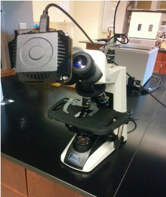
Figure 2. (a) Microscope used to measure fiber diameters using objectives of higher magnification. (b) Drawing apparatus comprising the tungsten tip fixed to a micromanipulator, thermocouple, microscope and the heater.
