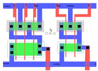
Figure 1. Sample of a 2input and 3input NAND logic gate for implemention in adiabatic circuits with 2 power clocks (PwrClk+ and PwrClk-)
