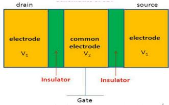
Figure 2. Single Electron Transistor (SET) layout.<sup>1</sup>
