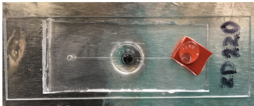
Figure 1: The experimental apparatus. A microfluidic channel connects the two volumes of electrolyte solution, right and center. The silicon nitride chip containing the drilled pore is affixed to the PDMS microfluidic through a process of oxygen plasma sealing and sequential heat treatment. The pore is located in the center of the black chip in the protein reservoir, center.
