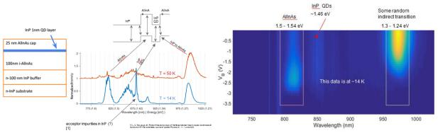
The image on the left is the spectra depicting the peaks with their wavelengths, and what transitions we think they are supposed to come from. The one on the right shows the experimental reading.
