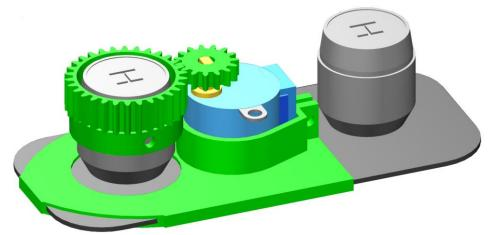
This image shows the setup we made with the 3D printer to connect the stepper motor to the knob on the laser.
