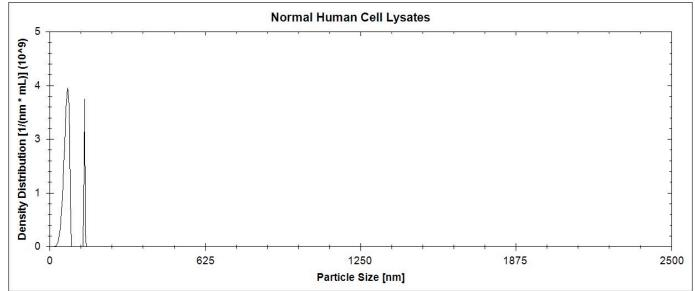
This is a graph taken from the LightSprite device depicting the particle size vs. density distribution curve from a dataset for normal (healthy) human cell lysates. The lysates show peaks of 72 and 141 nm, which represent particle sizes/diameters. Using the trapezoidal rule to find the
