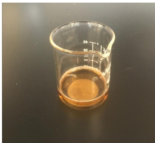
Figure 1. Beaker containing EDTA-free Pd bath solution, with Pd-coated disk inside
