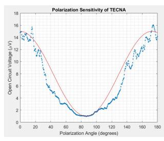
The result was an approximate cosine squared relationship which is consistent with antenna theory. The next steps are to continue building a dataset of these tests for different antennas with varying fabrication methods and in different environments such as a vacuum to continue to improve the sensitivity of the detectors.
