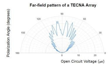
The signal peaks around 90 degrees which is where the H-field of the antenna is aligned with the magnetic field of the light (perpendicular angle). The surrounding 'fringes' of peaks are the result of constructive and destructive interference when light is reflected by the silicon substrate back to the antenna. Tests were also conducted with arrays where the antenna was off-centered from the cavity such that the peak would occur at other angles. When multiple of these
